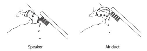
① Do not use anything sharp or excessive force while removing earwax or debris. The speaker and the air duct may be damaged.
